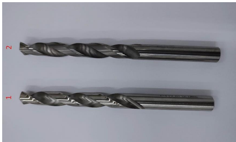
Figura 12 – Broca de HSS e Metal duro, vista lateral. 1 – Broca HSS. 2 – Broca Metal duro
