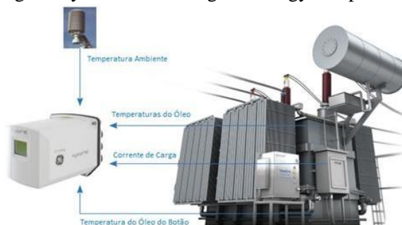
Fig. 2. Hydran M2 Ge Digital Energy Adaptado de [7]
