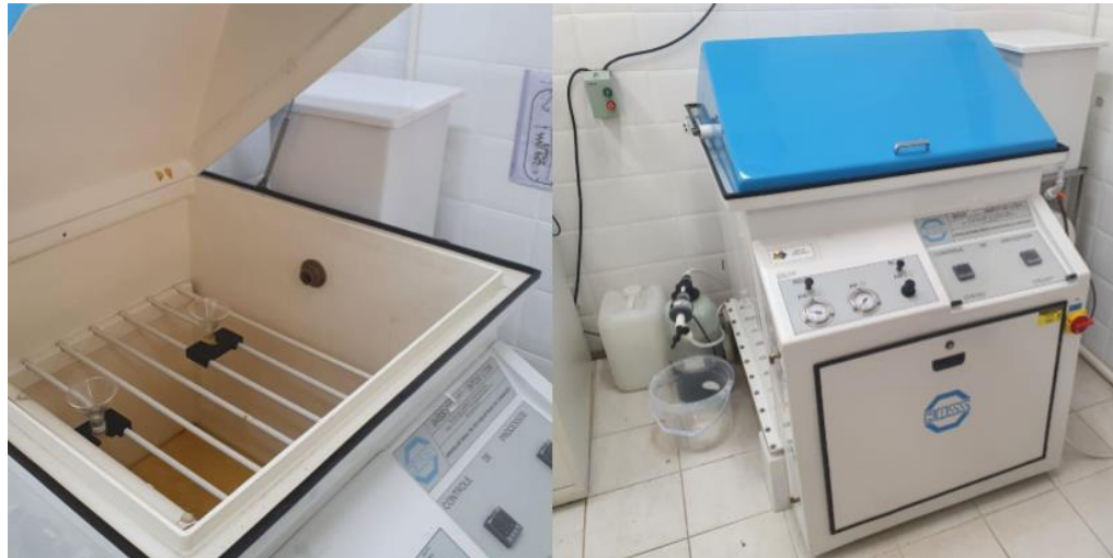
Figura 19 - Teste salt spray.
