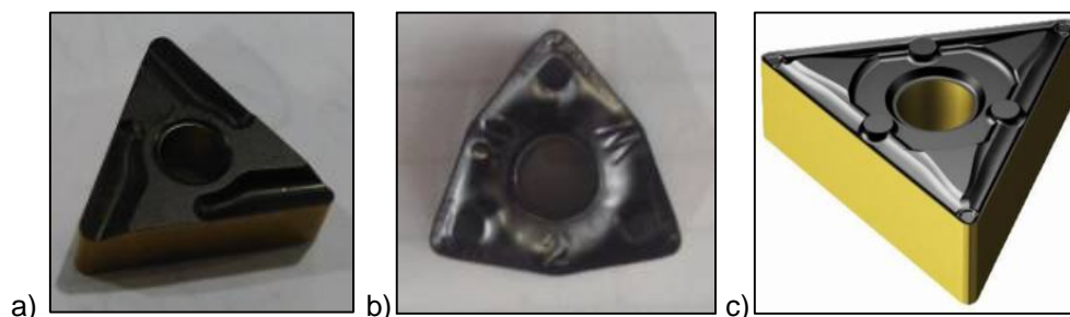
Figura 8 – a) geometria T standard , b) geometria W wiper , c) geometria T wiper .
