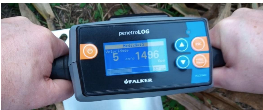
Figura 18 – Layout do penetroLOG ® .
