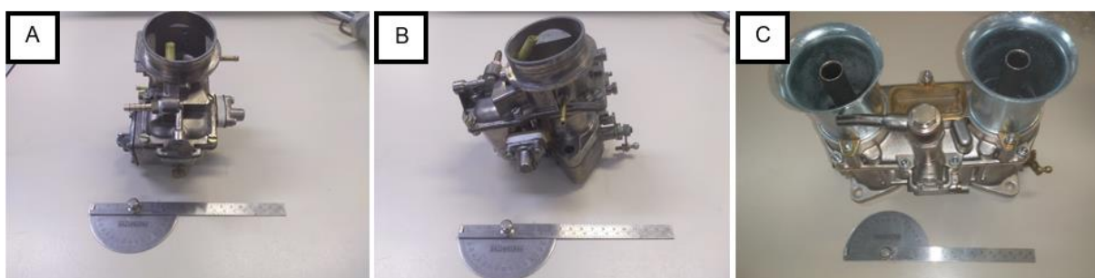
Figura 18 - Carburadores Solex 32(A), Solex 40(B) e Weber 48(C)
