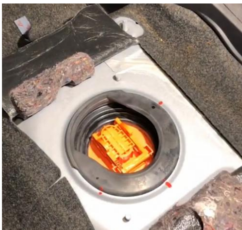
Figura 11 – High Voltage Disconnect (HVD)
