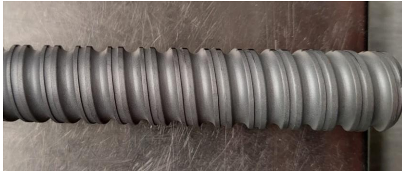
Figure 20 – Worm drive coated with sandblasting
