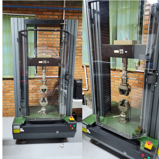
Figura 54: Computer Controlled Universal Testing Machine - Modelo WDW - 100 E
