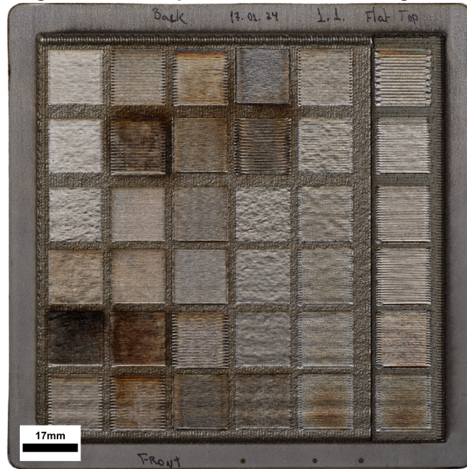
Figure 38 - Flat top with 36 remelted testing fields
