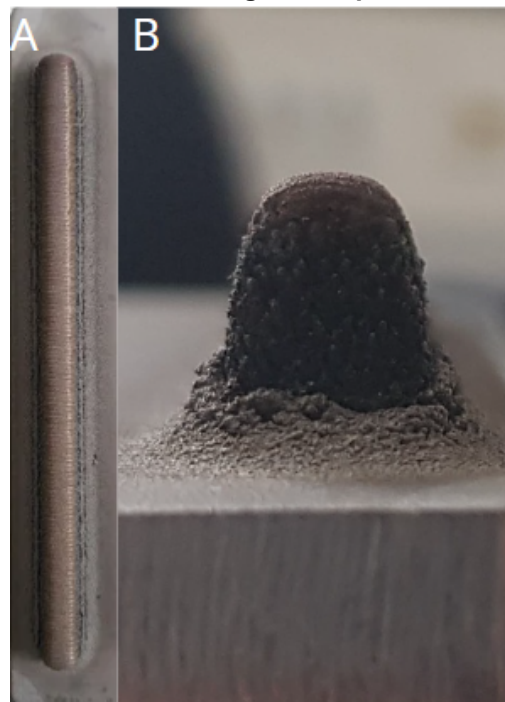
Figure 33 - A) Top view of the 90° cross-hatching wall deposition. B) Side view of the 90° cross-hatching wall deposition
