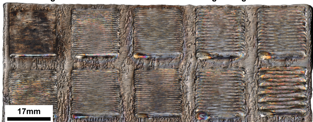
Figure 25 - Sandblasted Wall with Remelting testing fields
