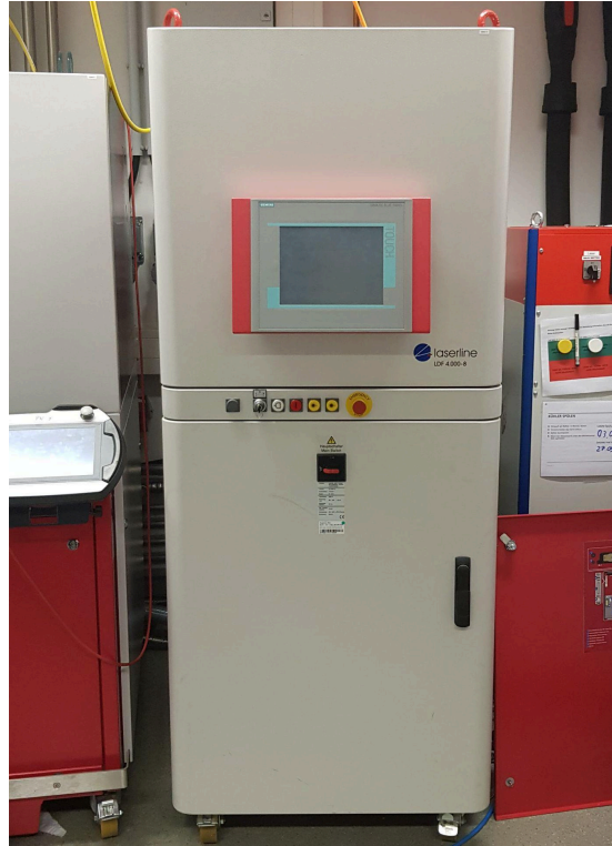
Figure 12 - Laser power supply LDF 4000-8
