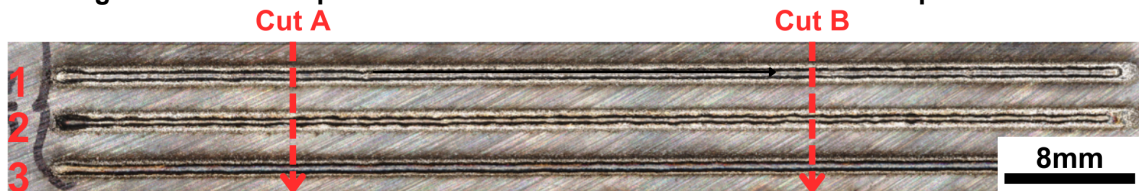
Figure 14 - Bead deposition on substrate and cross-section cuts representation
