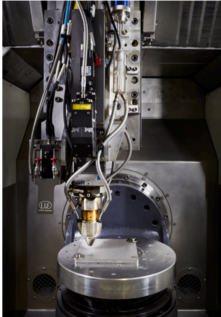
Figure 11 - Optical system installed in the CNC machine
