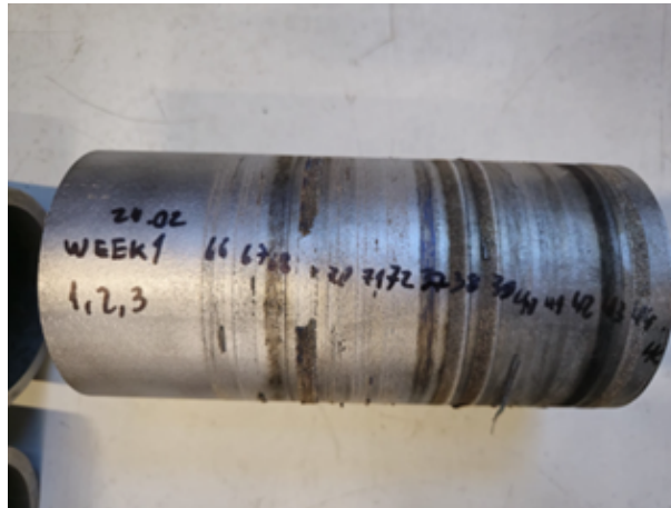
Figure 14 – Tube Week 1 - Lack of fusion
